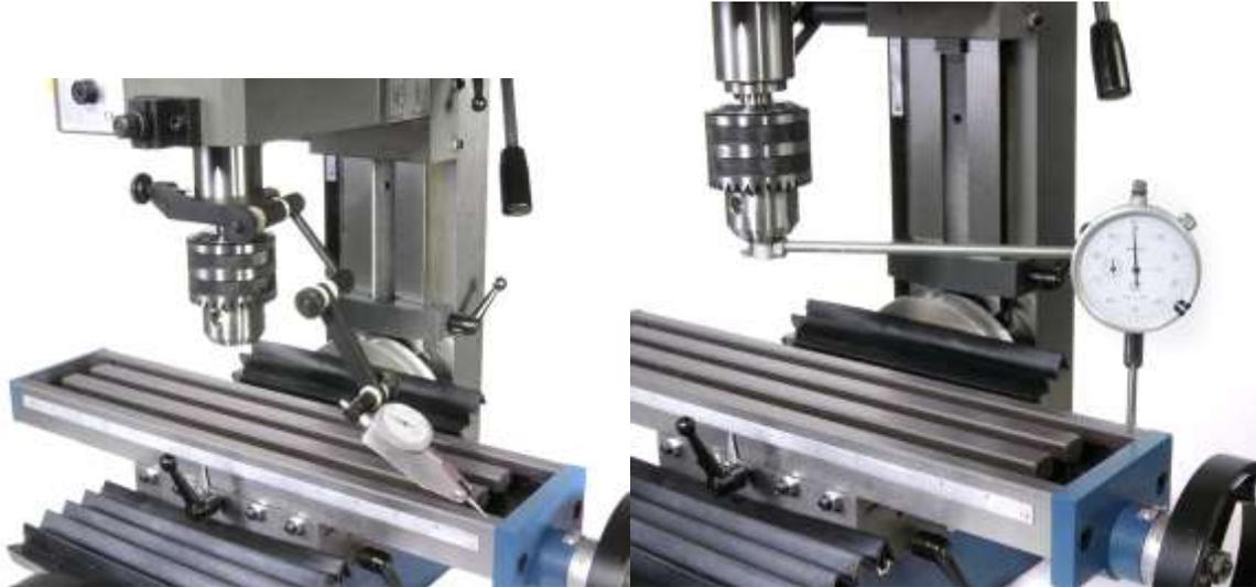
4. Take readings on the left front and right front corners of the table. Calculate the difference to see how much and which way to move the top of the column.
