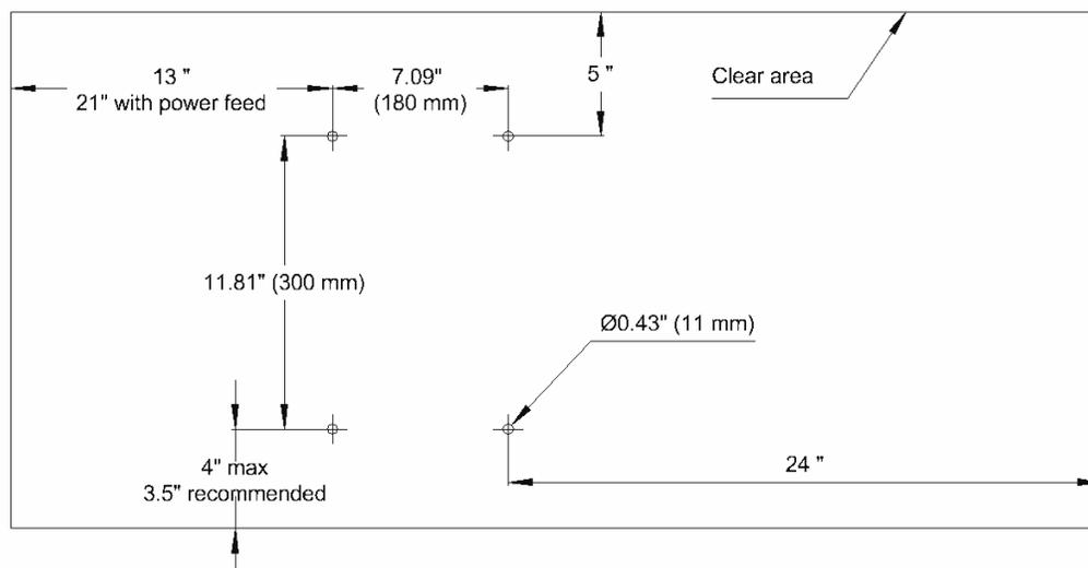
Mount the mill to the workbench with 3/8" or 10 mm bolts. The bolts should be about 1" (25 mm) longer than the thickness of the workbench. Use fender washers on the underside of wooden benches to prevent the nuts from pulling through.
