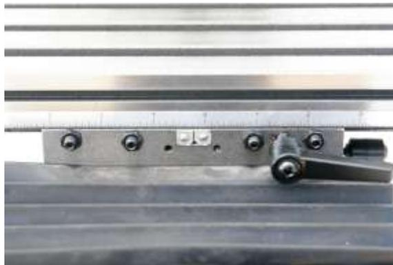
X-axis gib adjusting screws
