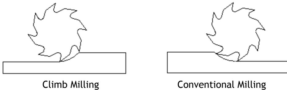
Depending on the direction in which you move the workpiece against the end mill you are either climb milling or conventional milling. As shown in the illustration above, you are climb milling when the end mill turns as to climb the slope made by cutting.
