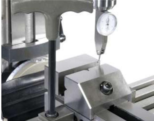
7. Move the Y-axis so that the dial test indicator's point contacts the fixed jaw of the vise. Continue moving the Y-axis to zero the dial test indicator.
